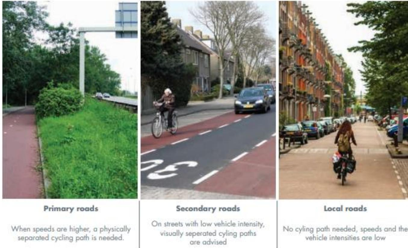
**Figure 8: the intensities of cycles and cars, and the speeds of the car determine the lay-out of the infrastructure.**
